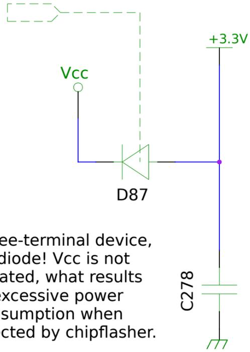
Three-terminal device, no diode! Vcc is not isolated, what results in excessive power consumption when injected by chipflasher.
